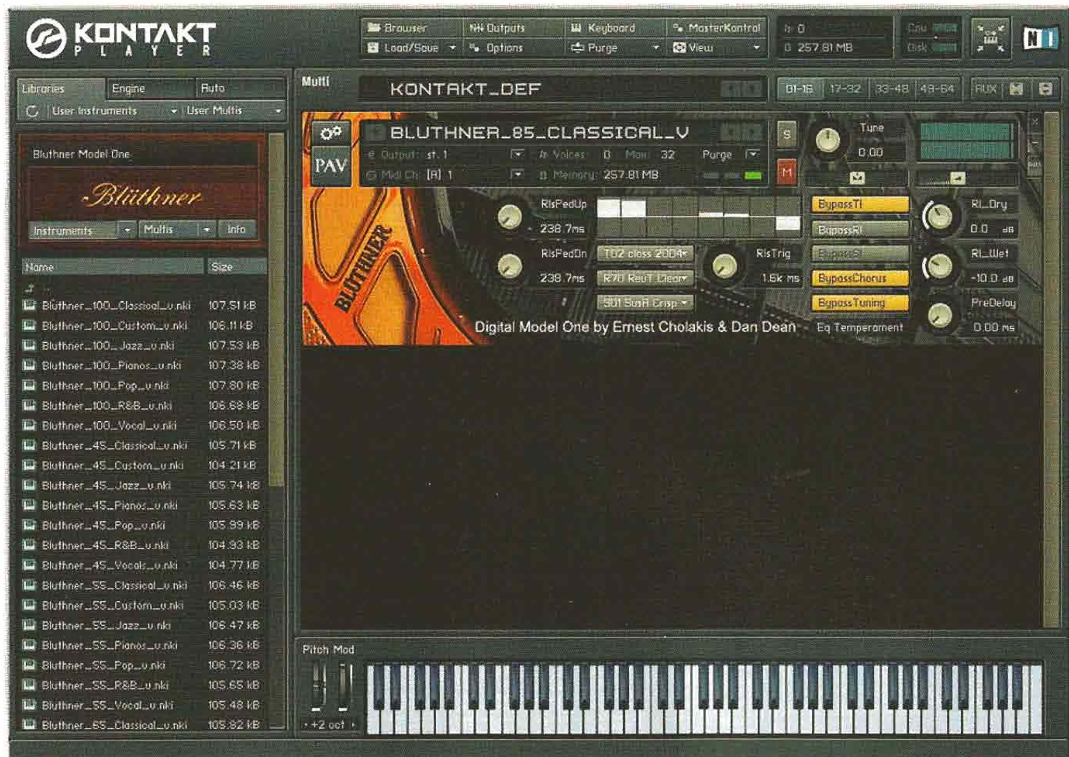
The Digital Model One's Kontakt 2-based interface allows easy access to all of the parameters of the instrument.
